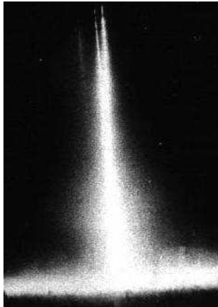
Fig. 12. The plasma impulse antennas created in the air by a hypervelocity Al body.
