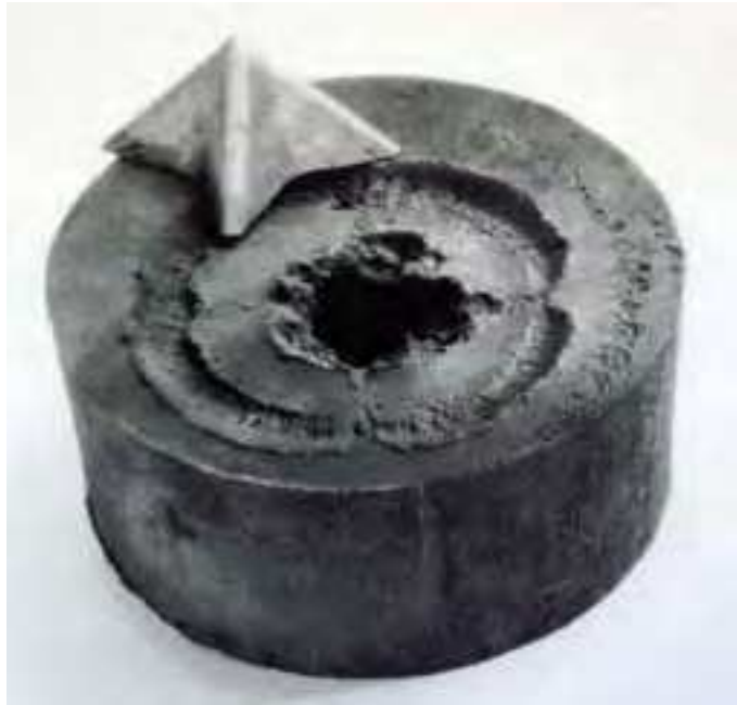
Fig. 18. Star-like liner for the shaped charge and the target.
